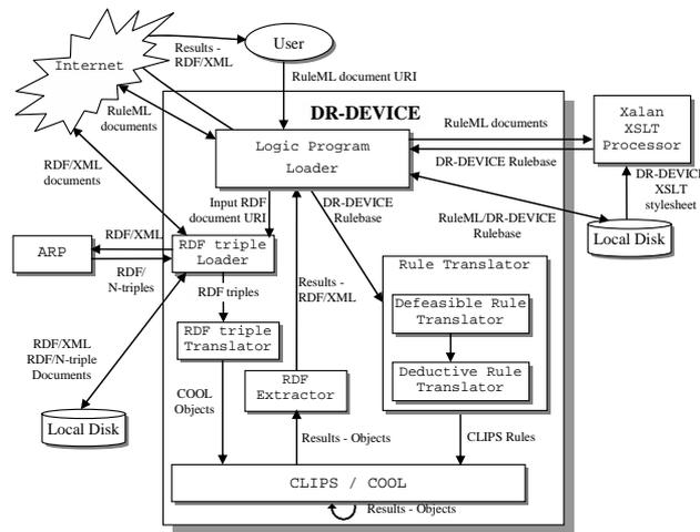
**Fig. 1.** Architecture of the DR-DEVICE reasoning system.
