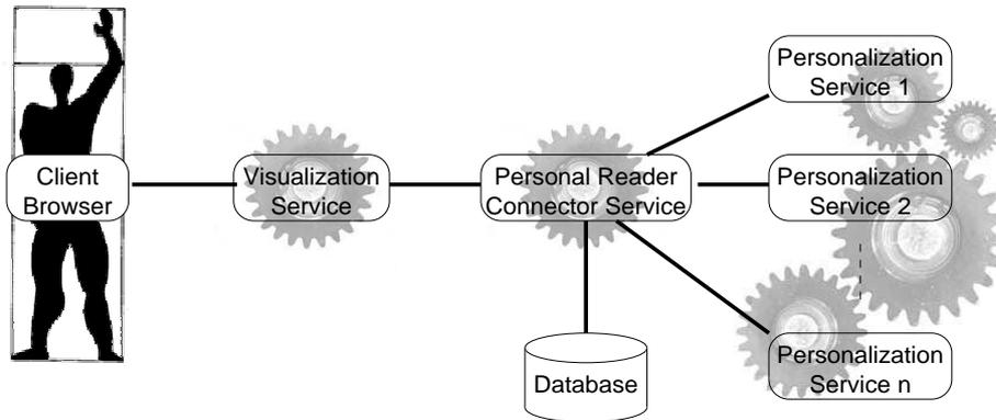
**Fig. 1.** Architecture of the Personal Reader framework, showing the different components of the Personal Reader: Visualization (user interface), the Personal Reader backbone (consisting of the Connector Services, the Reasoning Service(s)), and some data-provision services, for RDF data and for the connection with some database for storing user profile information.
